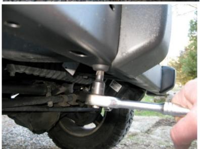
4. If not installing a winch and you would like to run fog lights install fog lights at this time. The tab will need to be bent flush (as shown in the photo)
