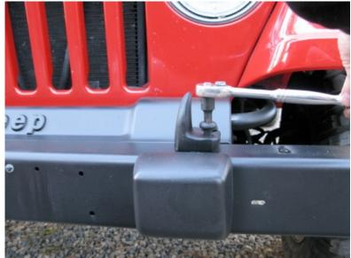
3. Remove the 2-T55 bolts on the bottom of bumper. (1 on each side)
