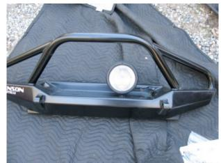
6. With the front bumper prepared and the stock bumper removed, place bumper on the end of the frame horns.
