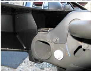
8. Two bolts mount on the topside of the frame and one installs on the underside.
