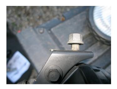
5. The factory fog lights can be installed in place of the winch as shown.
